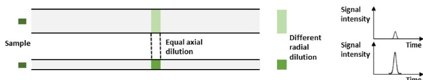
**Figure 1** – Illustration of radial dilution and the effect on signal intensity, on a conventional sized column (above) and miniaturized column (below).
