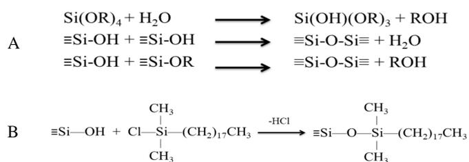
**Figure 2** – A: Overall reactions of the sol-gel process when a silicon alkoxide is used as monomer. B: A typical functionalization process where a C18 stationary phase is attached to silica.
