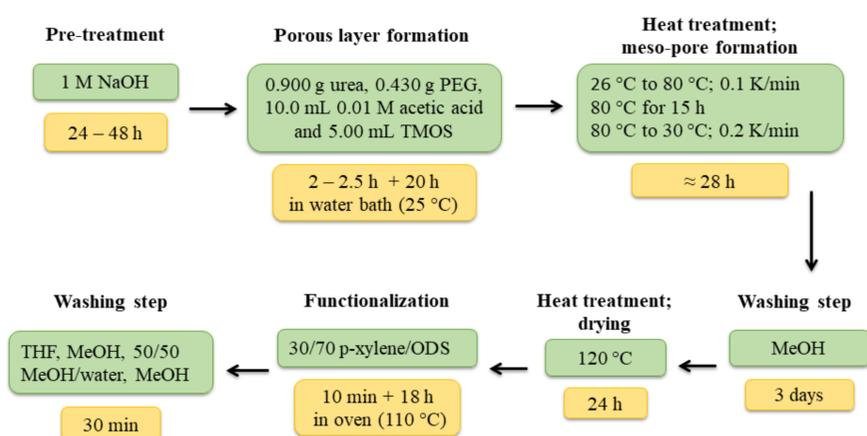
**Figure 3** – Overview of the PLOT column preparation process. TMOS: tetramethyl orthosilicate, PEG: polyethylene glycol, ODS: chloro(dimethyl)octadecylsilane
