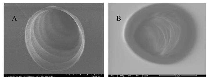
**Figure 5** – Scanning electron micrographs of a fused silica capillaries with successfully formed porous layer with 5  $\mu\text{m}$  ID (A) and 10  $\mu\text{m}$  ID (B).
