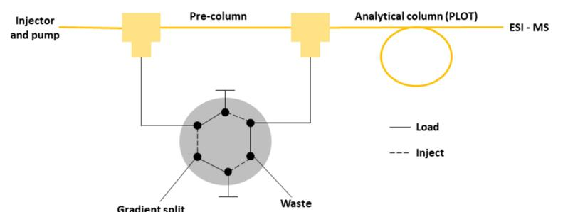
**Figure 4** – Schematic drawing of the chromatographic system used with PLOT column as analytical column. For analysis of a cytochrome C digest, an in-house made silica-based monolithic pre-column (C18, 50  $\mu\text{m}$  x 4 cm) was used, together with a 10  $\mu\text{m}$  ID silica-based C18 PLOT column (length between 115 and 120 cm). Mobile phase flow rate through PLOT column was 60 nL/min.
