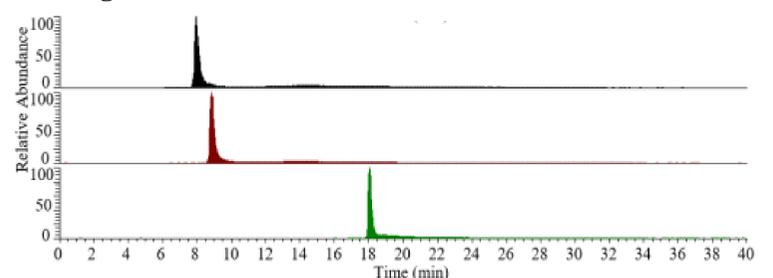
**Figure 6** – Extracted ion chromatogram for three different peptides from a cytochrome C digest, using a 10  $\mu\text{m}$  ID PLOT column with C18 stationary phase. The chromatographic system used is shown in **figure 4**. Mobile phase solution A: 0.1 % formic acid in water, B: 10% water and 0.1% formic acid in acetonitrile. The gradient used was 3-50 % B in 30 minutes.
